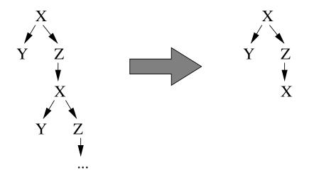
Observation: One can always find a *finite* prefix containing the same reachable states as the infinite unfolding (by unrolling loops exactly once). We shall call such a prefix complete.
