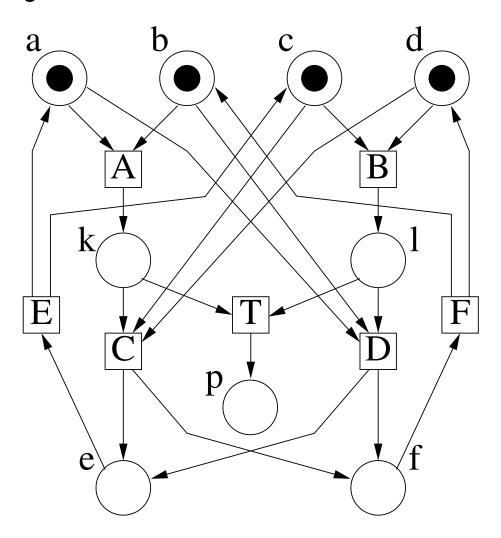
In Example 2 the marking  $\{p\}$  is reachable, e.g. by firing ABT.
