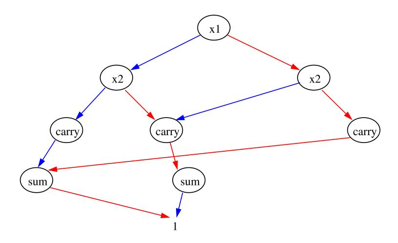
For a clearer graphical representation, one can remove the 0-node  $\rightarrow$  missing edges implicitly lead to 0
