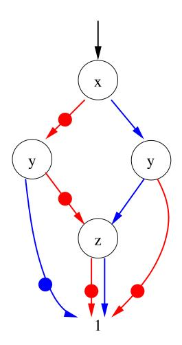
For this reason, the *z*-labelled node is *not redundant*. The **0**-leaf can be omitted altogether.
