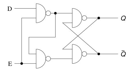
controls **D** (data) and **E** (enable):
