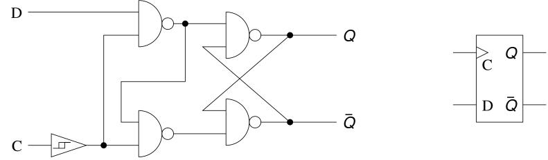
In block diagrams, *C* is distinguished by a triangle.
