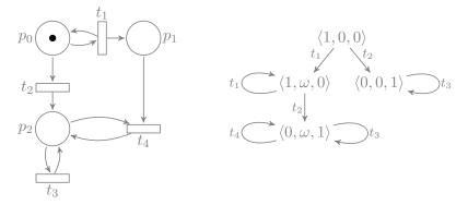
Its coverability graph has a *decreasing* cycle on  $(0, \omega, 1)$  when firing  $t_4$ .
