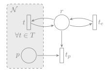
Assume that  $m_0 \to_{\mathcal{N}}^* m$  with m(p) = 0. Then the same sequence of transitions can be fired in  $\mathcal{N}'$ , leading to  $m_0 \oplus r \to_{\mathcal{N}'}^* m \oplus r$ , from which  $t_e$  can be fired infinitely often: this constructs an infinite execution of  $\mathcal{N}$  where  $t_p$  is infinitely often not firable, i.e. a weakly fair execution for  $t_p$ .
