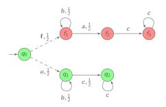
$\checkmark$  c is surely correct since  $\mathcal{P}^{-1}(c) = \{q_0uq_1cq_2\}.$  $\checkmark$  ac is surely faulty since  $\mathcal{P}^{-1}(ac) = \{q_0ff_1af_2cf_3\}.$
