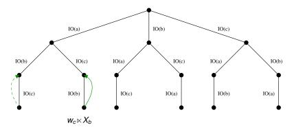
P = IO(a)|IO(b)|IO(c) where  $IO(I) = in(c_I, X_I).out(c_I, w_I)$
