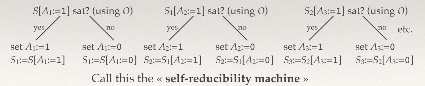
Instead of an oracle O, Merlin will use circuits C<sub>m</sub> on clause sets S, S<sub>1</sub>, S<sub>2</sub>, ..., of various sizes m.
