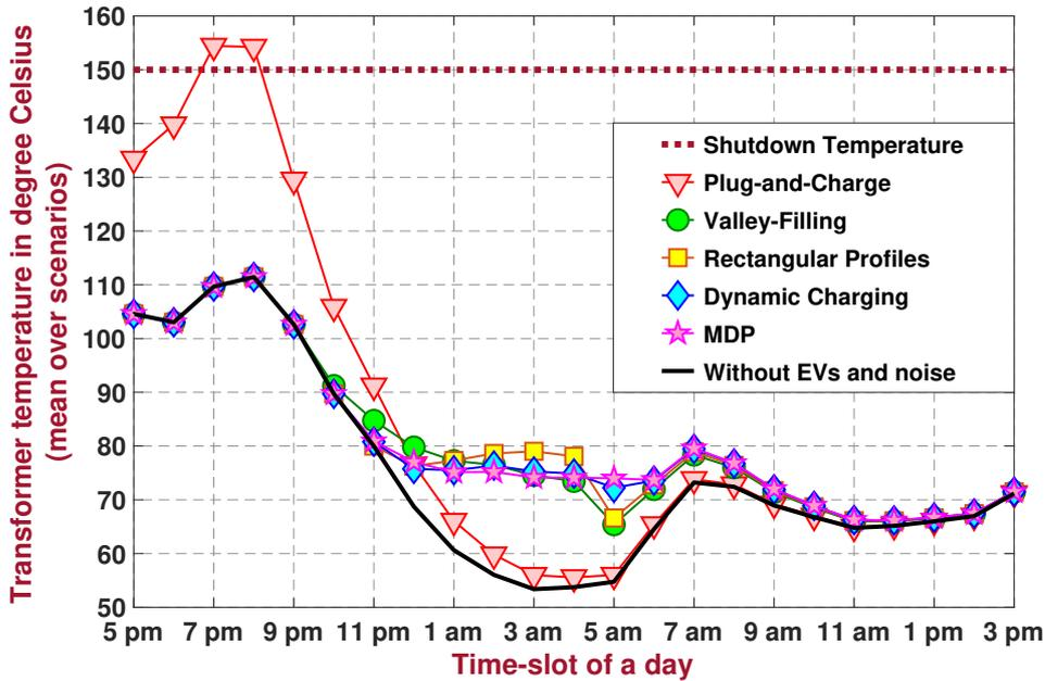
Figure 3.8: HS temperature of the DN-transformer (mean over the scenarios) for  $I = 10$  EVs over time, based on a forecast of the noncontrollable consumption with a noise (in each scenario) based on  $\text{SNR} = 15 \text{ dB}$  (centralized case).
