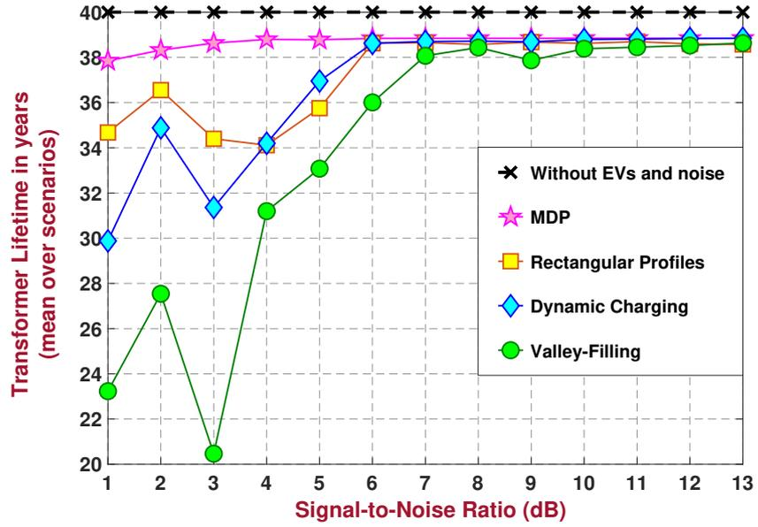
Figure 3.9: DN-transformer lifetime (mean over the scenarios) against forecast noises on the noncontrollable consumption, for  $I = 10$  EVs (centralized case).
