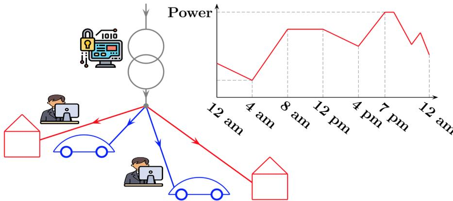
Figure 6.1: A typical scenario which is captured by the model analyzed in this chapter. Each EV controls its charging power profile to reach its demanded state of charge, for instance for its next trip. The charging consumption is based on some coordination mechanism among the EVs and some knowledge about the day-ahead (aggregated) noncontrollable part of the total consumption.
