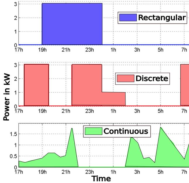
Figure 3.2: Four charging models of an EV: rectangular, continuous and discrete charging. Each model corresponds to a class of electrical uses far broader than the case of EVs.
