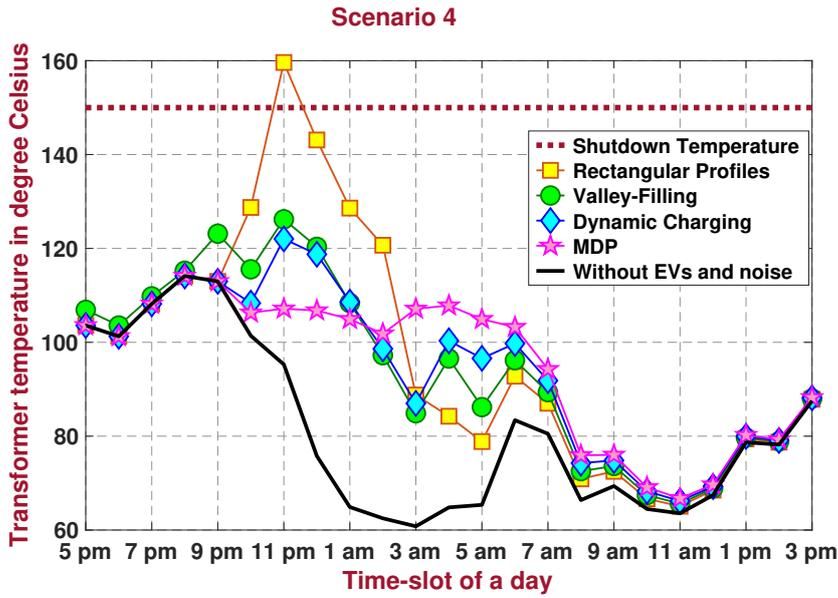
Figure 3.11: HS temperature of the DN-transformer (mean over the scenarios) for  $I = 20$  EVs over time, based on a forecast of the noncontrollable consumption with a noise (in each scenario) based on  $SNR = 6$  dB (centralized case).
