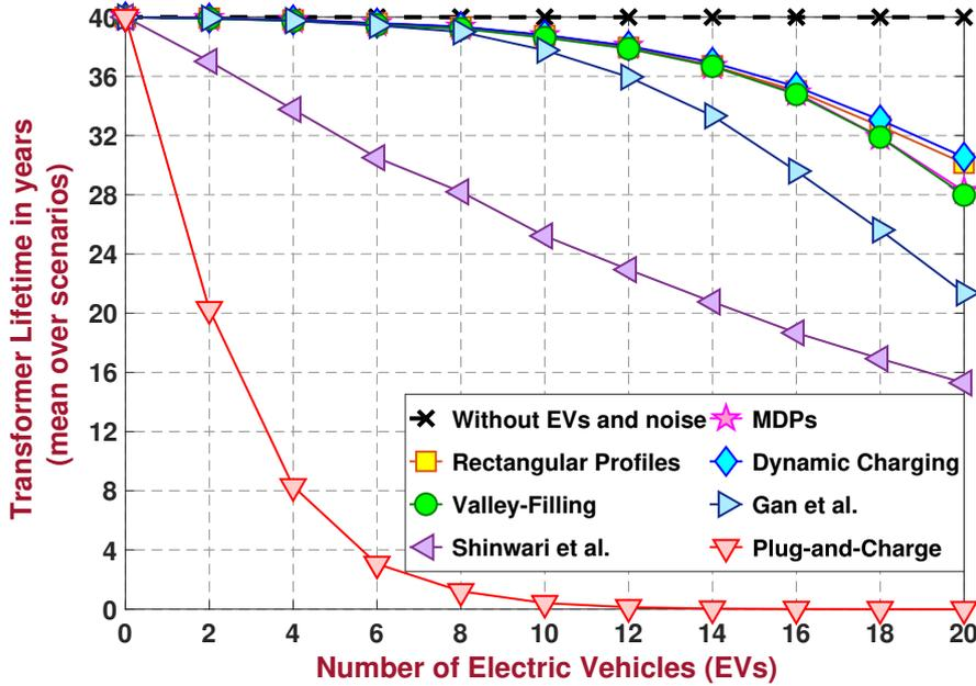
Figure 6.5: DN-transformer lifetime (mean over the scenarios) against the number of EVs ( $I$ ), based on a forecast of the noncontrollable consumption with a noise (in each scenario) based on  $\text{SNR} = 15 \text{ dB}$  (decentralized case).
