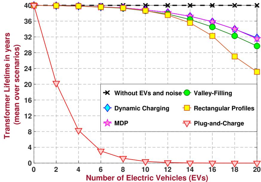
Figure 3.7: DN-transformer lifetime (mean over the scenarios) against the number of EVs ( $I$ ), based on a forecast of the noncontrollable consumption with a noise (in each scenario) based on  $\text{SNR} = 15 \text{ dB}$  (centralized case).
