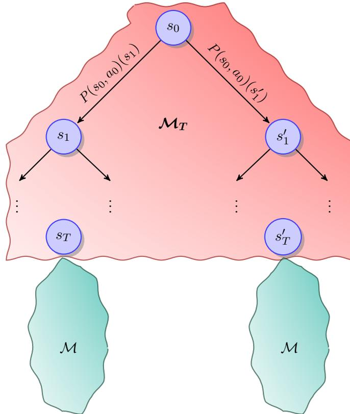
Figure 4.4: Unfolding  $\mathcal{M}_T$  of the MDP  $\mathcal{M}$ , where we keep a copy of  $\mathcal{M}$  below each leaf  $s_T$ .
