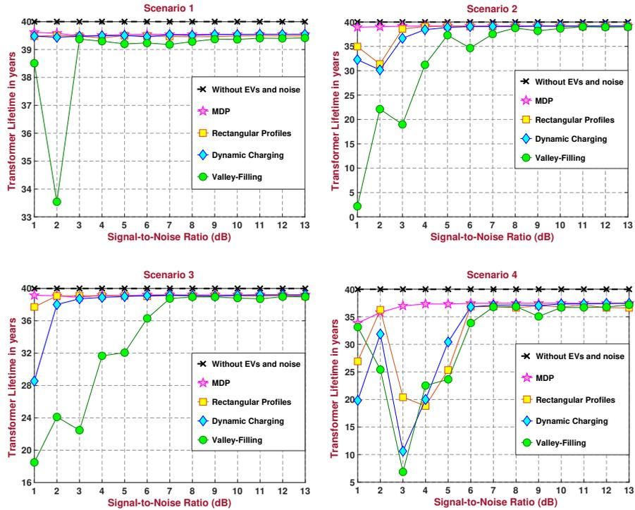
Figure 3.10: DN-transformer lifetime (in each scenario) against forecast noises on the noncontrollable consumption, for  $I = 10$  EVs (centralized case).
