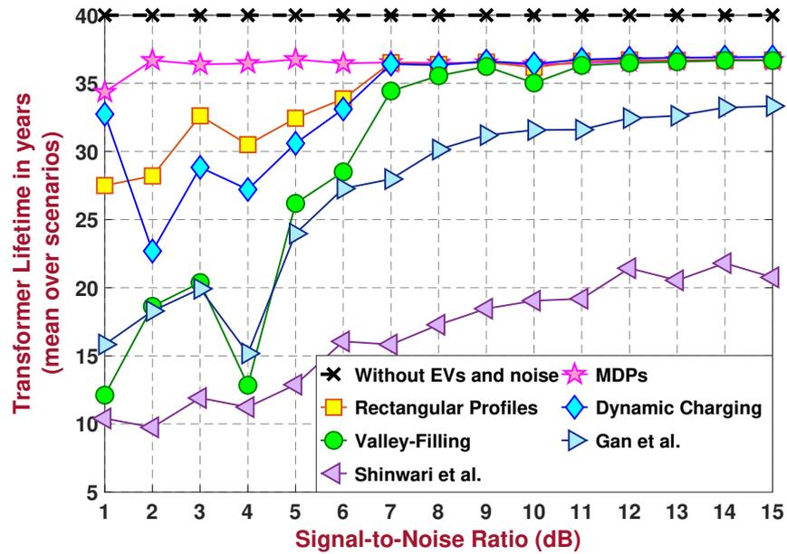
Figure 6.6: DN-transformer lifetime (mean over scenarios) against forecast noises of the noncontrollable consumption, for  $I = 15$  EVs (decentralized case).
