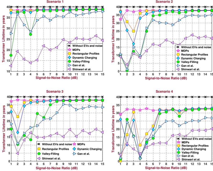
Figure 6.7: DN-transformer lifetime (in each scenario) against forecast noises on the noncontrollable consumption, for  $I = 15$  EVs (decentralized case).
