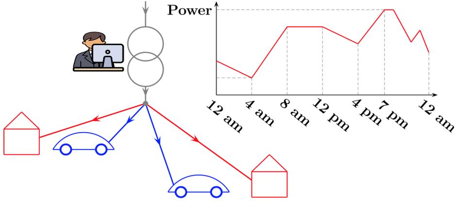
Figure 3.1: A centralized decision-maker controls the charging power of EVs to reach the individual energy demands. The centralized scheduler have some knowledge about the day-ahead (aggregated) noncontrollable part of the total consumption.
