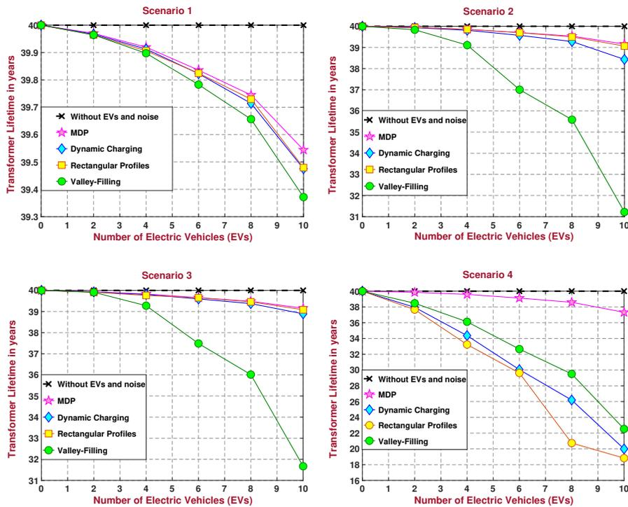
Figure 3.12: DN-transformer lifetime (in each scenario) against the number of EVs, for a forecast noise based  $SNR = 5$  dB (centralized case).
