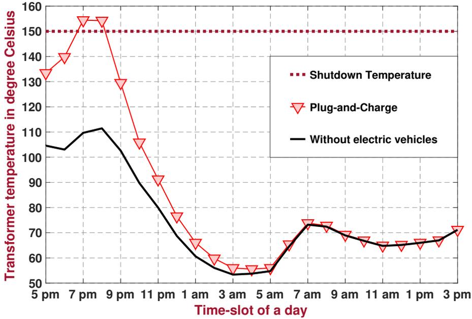
Figure 2.2: Impact of the charging scheme Plug-and-Charge (PaC) on the evolution of the DN-transformer Hot-Spot (HS) temperature, under the assumption of  $I = 10$  Electric Vehicles (EVs). In this case, the shutdown temperature is exceeded for such a method of charging. (the HS model used was the one of [19] and the real data was taken from [3]).
