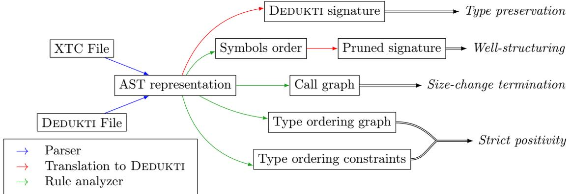
Figure 1: SIZECHANGETOOL Workflow
