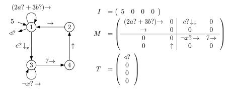
Each accepting run of  $\mathcal{A}$  over u has weight  $5 \times 2^{|u|_a} \times 3^{|u|_b} \times 7^{|u|_c}$
