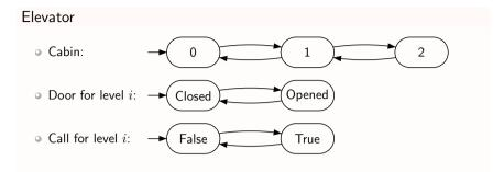
The actual system is a synchronized product of all these automata. It consists of (at most)  $3 \times 2^3 \times 2^3 = 192$  states.
