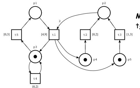
Initial marking:  $(p_1, p_2(2))$ Only  $t_1$  can be fired:  $4 \le t_1 \le 9$   $\rightarrow t_1$  is fired after  $\theta_1$ Marking:  $(p_3, p_4, p_5)$   $t_2, t_3, t_4$  and  $t_5$  can be fired:  $0 \le t_2 \le 2$   $0 \le t_3 \le 3$   $0 \le t_4 \le 2$   $0 \le t_5 \le 3$  $\rightarrow t_2$  is fired after  $\theta_2$
