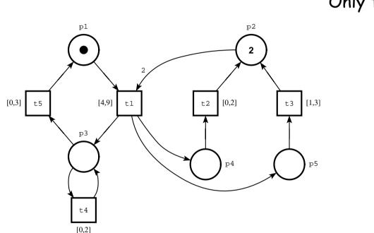
**Initial marking:**  $(p_1, p_2(2))$ Only  $t_1$  can be fired:  $4 \le t_1 \le 9$  $\rightarrow t_1$  is fired after  $\theta_1$
