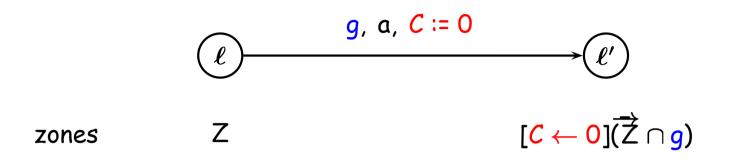
A zone is a set of valuations defined by a clock constraint
