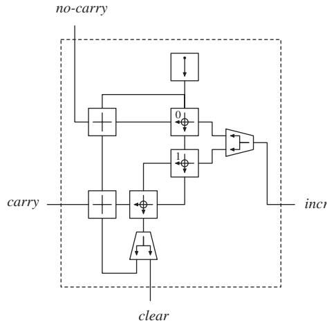
Fig. 13. Symbolic diagram of a bit device.
