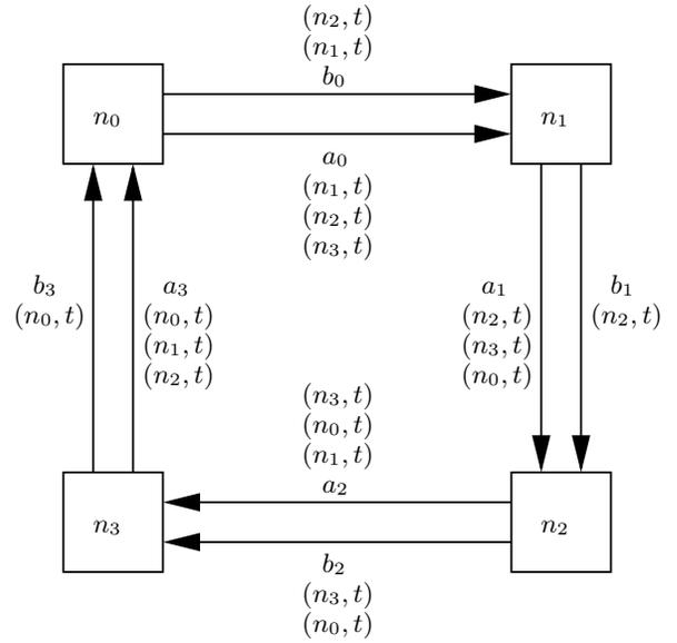
Fig. 3. The interconnect with all edges labeled with messages transiting through channels
