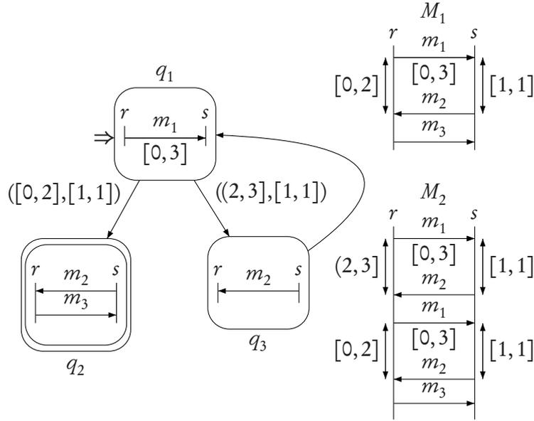
Figure 5: A TC-MSG and some TC-MSCs that it generates
