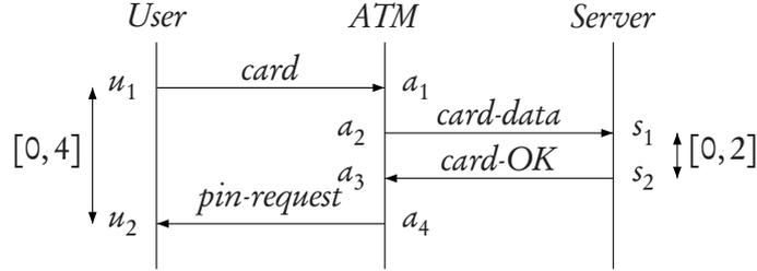
**Figure 2:** A TC-MSD describing interaction with an ATM.
