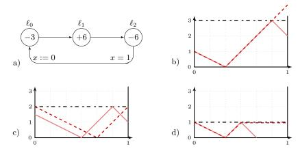
**Fig. 1.** a) Weighted Timed Automaton (global invariant  $x \le 1$ ). b)  $U = +\infty$  and U = 3. c) U = 2. d) U = 1 and W = 1.
