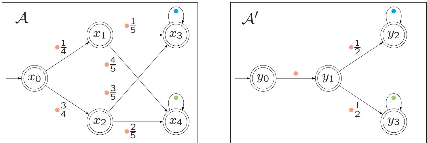
$$\phi^* \equiv \begin{cases} x_0 = y_0 \\ \frac{x_1}{5} + \frac{3x_2}{5} = \frac{y_1}{2} \\ \frac{4x_1}{5} + \frac{2x_2}{5} = \frac{y_1}{2} \\ x_3 = y_2 \\ x_4 = y_3 \end{cases} \quad \wedge \quad \begin{array}{l} \sum x_i = \sum y_i = 1 \\ x_i, y_i \geq 0 \end{array}$$
